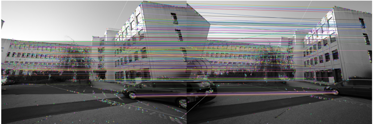
Figure 3.1: Salient points and matches between two images. In every image, salient points and feature descriptors are calculated using the SIFT algorithm. The corresponding feature descriptors are matched (connected with lines in this figure). As you can see, there exist some false matches, which can be eliminated using the Random Sample Consensus (RANSAC) algorithm in following steps.
