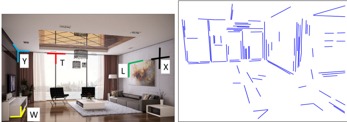
Figure 2.1: Identifying geometry by line segments. In [39], according to the appearance of a junction similar to a letter, the junctions are classified in types like L , T , Y , X . Using this information, it is possible to reconstruct the geometry of an indoor scene (left). Similarly, in [31] line segments are used to build geometry prototypes of indoor environments (right).
