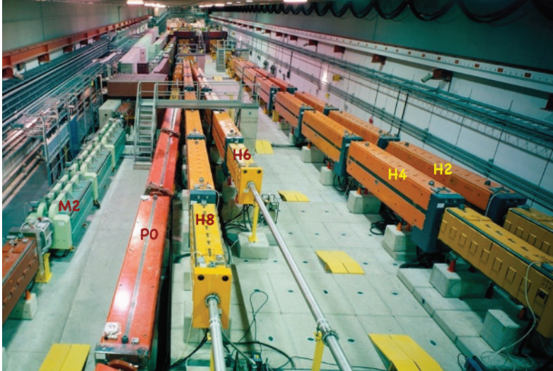
Figure 2: View of the H8 and other beam-lines emerging from the primary (T4) target located at the North Area test beam facility. [7]
