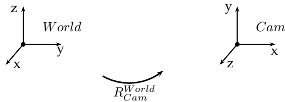
Figure 2.10: Illustration of the Nao coordinate frame rotation (left) and the usual computer vision notation (right). The rotation matrix \mathbf{R}_{\text{Cam}}^{\text{World}} can be calculated easily. Note, that the origin of both coordinate frames is the same.
