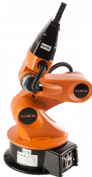
Figure A.5.: The Kuka YouBot manipulator. The image is taken from http://www.youbot-store.com/youbot-store/youbots/products/kuka-youbot-5-degree-of-freedom-arm-with-2-finger-gripper .
