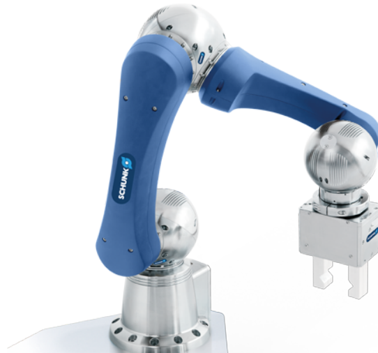
Figure A.7.: The Schunk Powerball manipulator. The image is taken from http://mobile.schunk-microsite.com/?id=9 .
