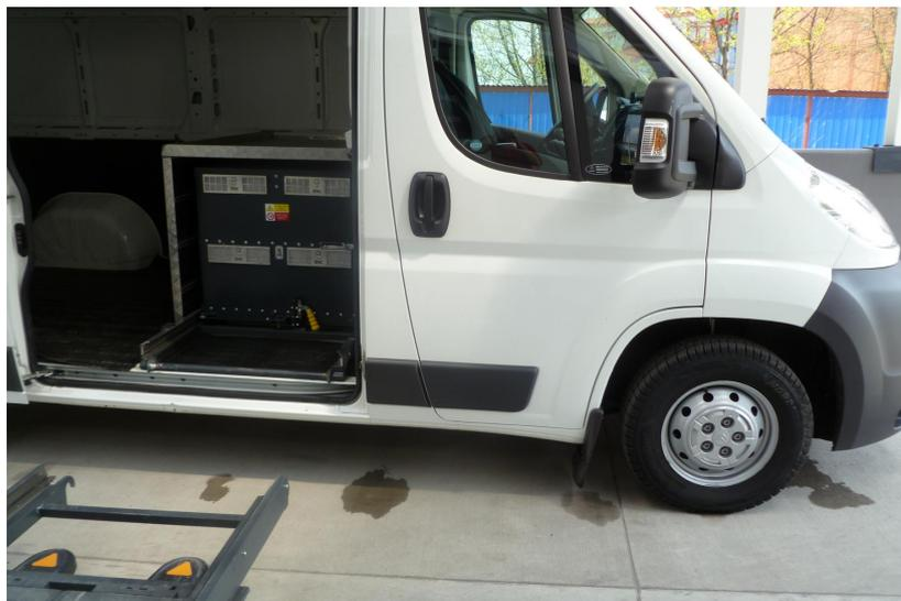
Figure 1.1: The electrically driven transporter designed for parcel delivering fleets, including a scenario of a battery exchange.
