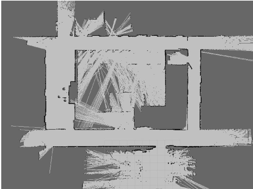
Figure 6.1: The figure represents the floor plan of the institute. Most of the base experiments took place there. It is generated through the usage of Gmapping, while exploring the floor with the robot steered through a game pad. The black pixel state obstacles, whereas light grey states free space. The dark grey parts are unexplored space but should never be tackled within our experiments.
