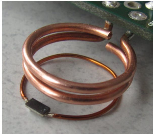
Figure 3.27: 868 MHz Loop antenna soldered onto PCB with tag underneath
