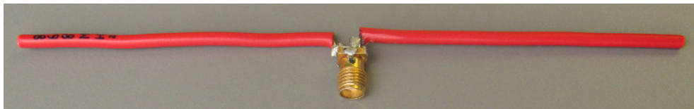
Figure 3.24: Dipole antenna for 868 MHz with SMA connector
