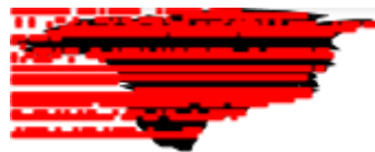
Figure 4.113.: Raphaël's original isPointInsidePath utility method does not work as expected, as shown in this test case, taken from (Martins, 2013). It illustrates isPointInsidePath results (red squares) when sampling a closed path (black shape).
