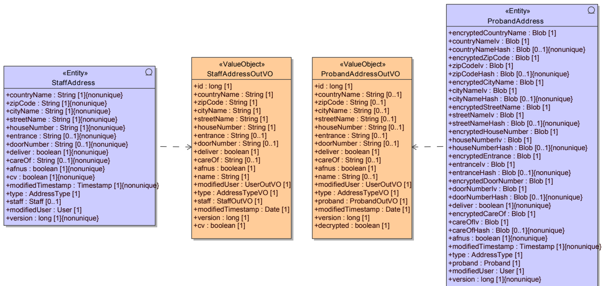
Figure 4.18.: Entities like StaffAddress and ProbandAddress are expected to qualify for ORM inheritance when looking at their mostly identical OutVOs. However, column encryption thwarts generalisation since it requires multiple entity fields in ProbandAddress per corresponding field of StaffAddress .
