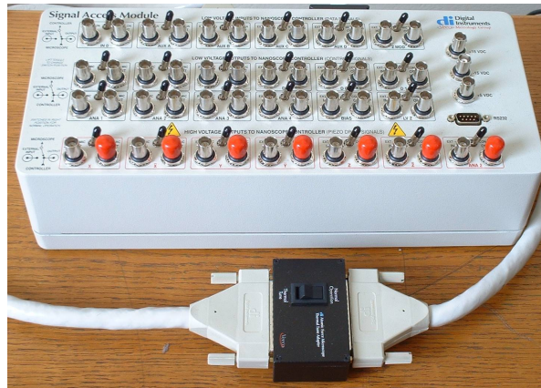
Figure 1.39: Signal access box to plug in the coaxial wires for applying some voltage to the active sample holder.
