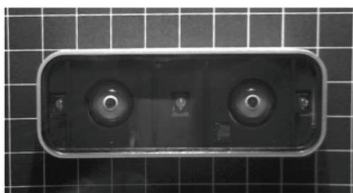
Image 7 - Leap Motion, LEDs and Cameras
