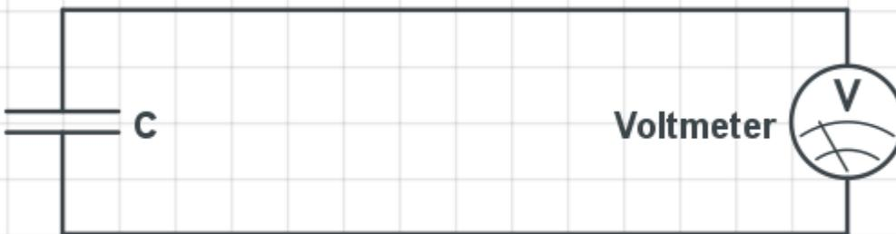
*Illustration 42: Analog model of pure oxygen sensor. The voltage stays the same.*
