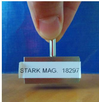
Fig. 1.2: Non magnetic steel sample with  $\mu_r \leq 2.5$  lifted up by a permanent magnet.
