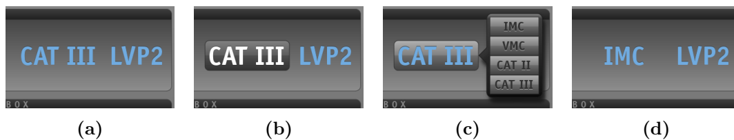
Figure 5.8: These images show a sequence of the button behavior implemented for the Parchim Airport system, where a button shall only be visible if necessary, i.e., when interaction is needed.
