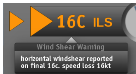
Figure 5.5: A windshear pop-up that fades in, when windshear conditions are serious and fades out if the wind conditions improve.
