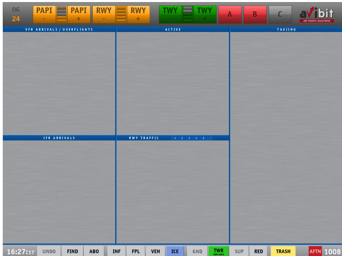
Figure 5.7: Integration of the airfield lighting control bar, shown at the bottom of Figure 5.6, as a separate application, on the screen of another system. Aside from the graphical differences in the user interface components, the removal of window decorations suggests one integrated system, instead of two separate ones.
