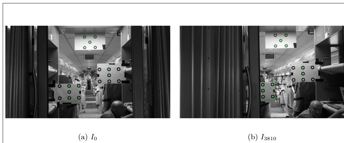
Figure 5.32.: (a) and (b) show frames with the carbodies in initial pose ( I_0 ) and at maximum displacement into y-direction at I_{3810} (compare to Figure 5.31b). Note the partial occlusion of T_2 by the gaiter of corridor connection. The tracking results are superimposed as green crosses.
