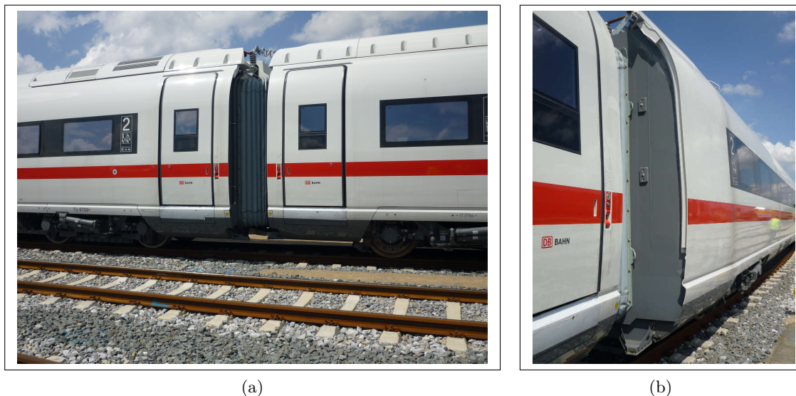
Figure 5.31.: (a) shows an outside view of the two selected carriages of the Siemens Velaro D which are linked by a flexible corridor connection. (b) pictures the carriages during relative displacement into y-direction.
