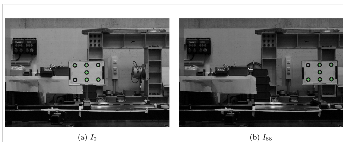
Figure 5.6.: (a) and (b) show frames recorded at beginning ( I_0 ) and maximum ( I_{88} ) of linear target displacement along y -axis. Although using less distance between camera and target, compared to Experiment 1a, the appearance of the target is smaller due to the shorter focal length applied. The tracking results are superimposed as green crosses.
