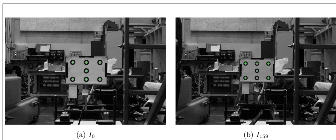
Figure 5.2.: (a) and (b) show frames recorded at beginning ( I_0 ) and end ( I_{159} ) of linear target displacement along x-axis performed in Experiment 1a. The tracking results are superimposed with green crosses.
