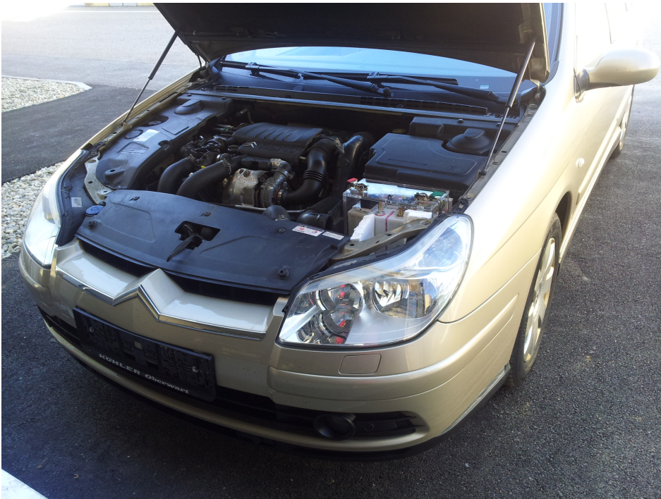
Figure 7.2: Citroen C5 with replacement battery installed
