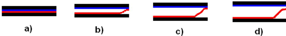
Figure 3.6: Illustration of a detaching process during a tensile test. a) Connected films. b) Sample gets stretched. One film starts to go adrift. c) The detaching process continues, while the films themselves are still connected. d) Films disconnect.
