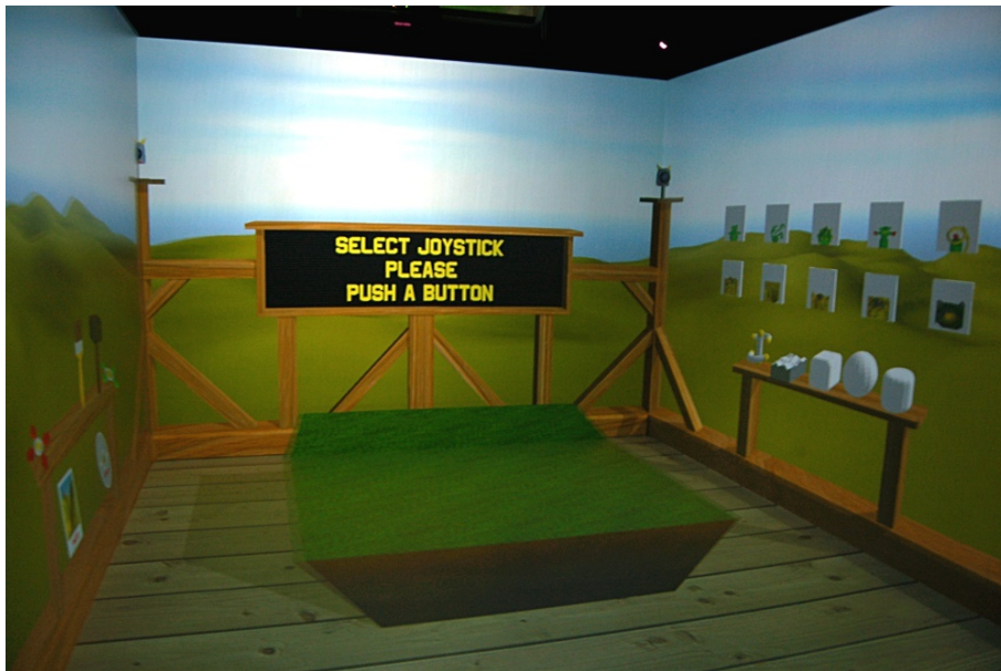
Figure 4.7: This photograph shows the modelling application right after it has been started. The info screen instructs the user to select a joystick by pressing a button. This step is necessary as multiple joysticks can be connected to the master computer simultaneously. As soon as the user complies, objects can be created and manipulated. By default, the landscape modelling tool is activated, recognisable by the flat green surface.
