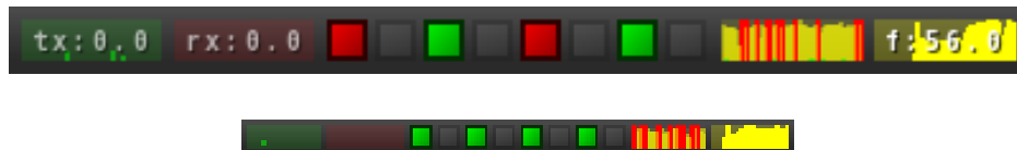
Figure 3.7: Two different screenshots showing the info bar. The bar will try to adapt to the application’s window size. In case the width of the window is smaller than 320 pixels, a more compact mode will be activated. In order to maintain a reasonable layout, each object has to be modified in both size and detail. A graph for example no longer displays its caption in order to reduce the required space.
