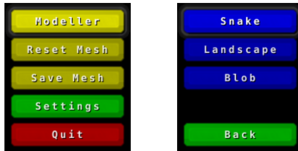
Figure 3.5: Two screenshots depicting the main menu. By selecting the Modeller button, a sub menu appears. Different colours immediately show which elements belong together. These menus do not require a large amount of space, hence all elements will be visible even at low screen resolutions.
