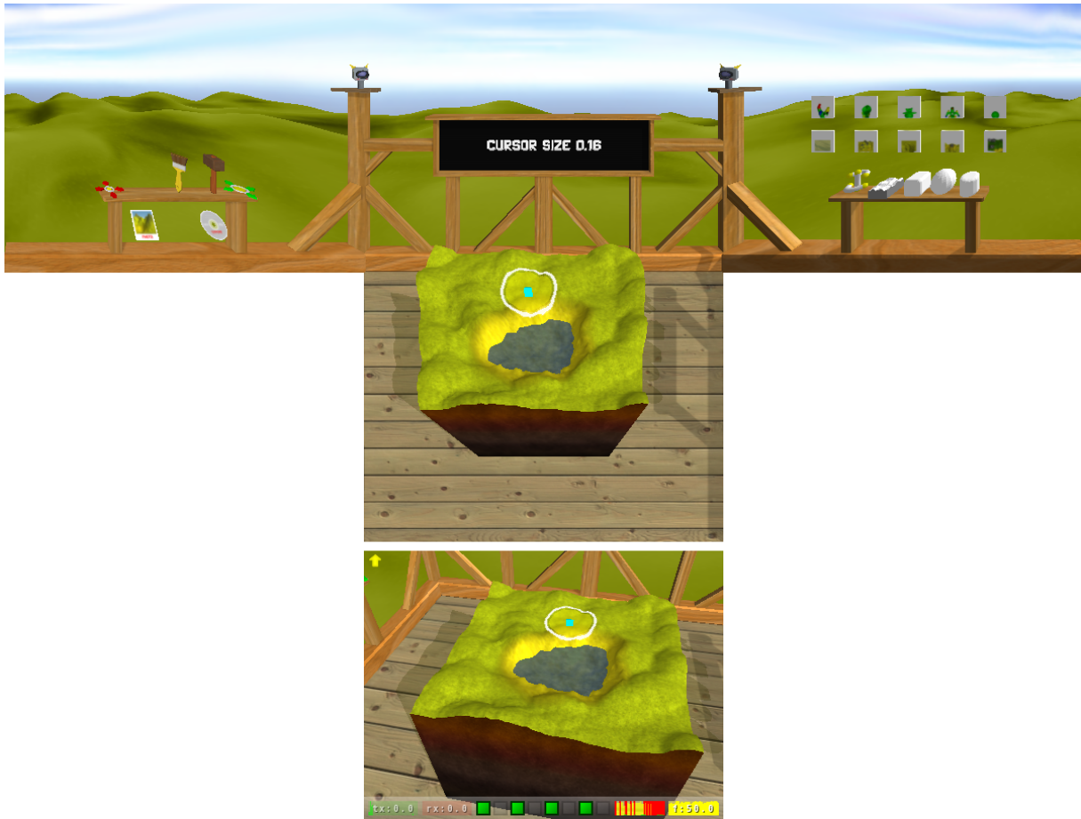
Figure 3.2: DAVE simulation using full mode . The image on the bottom shows the master application from the user's point of view. The remaining four applications represent the DAVE 's three walls and the floor. The images are distorted in order to produce a realistic environment from the user's point of view. By removing the window decoration, the applications merge to one seamlessly connected image. Each window is running at a resolution of 640x400 pixels with the double_size configuration parameter activated. The rendering process is rather time-consuming, the framerate is as low as 50 per second. Therefore the draw load graph, the second graph from right, is signalling a too long draw time, recognisable by the red colour. The computer that was used to create this screenshot simply was not fast enough. Nevertheless, the applications were still quite responsive.
