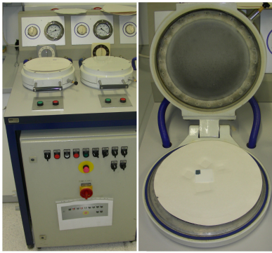
Figure 2.4: The sheet drier, the right side shows a typical sample arrangement on teflon and paper sheets.
