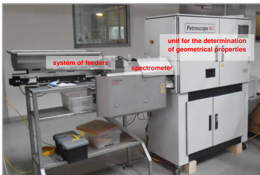
Fig. 9: Functional units of the measuring device Petroscope 4D ® .
