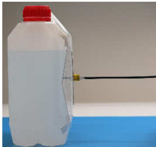
Figure 3.6: Measurement setup: The antenna with its measurement cables is mounted on the can filled with water.
