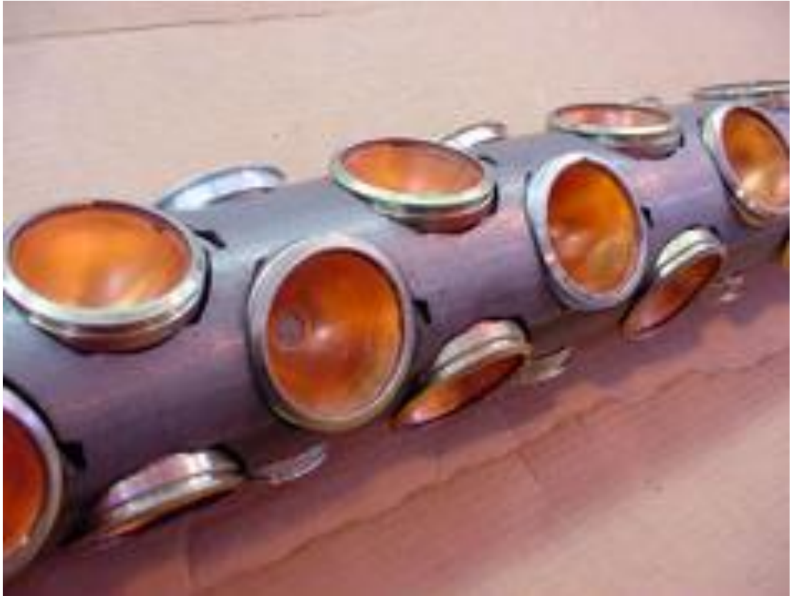
Abb. 30: Hohlladungsperforator (XL Perforating Partnership)
