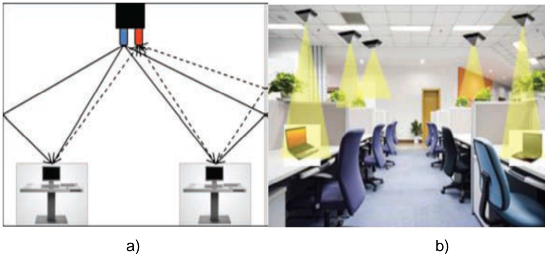
Fig.14. Optical wireless LANs: a) diffuse link and b) line of sight [6]
