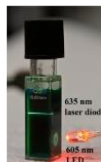
Figure 24 Solution of sensitizer (Palladium(II) 2,3-bis(3,3,9,9-tetramethyl-2-hydroxyjulolidine) but-2-enedinitrile and annihilator (diisobutyl 3,9-peryleneedicarboxylate) in deoxygenated toluene upon excitation with a 635 nm laser diode and LED [116]
