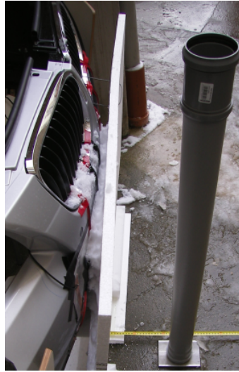
(a) Photograph of the measurement setup with a layer of snow in front of the bumper.
