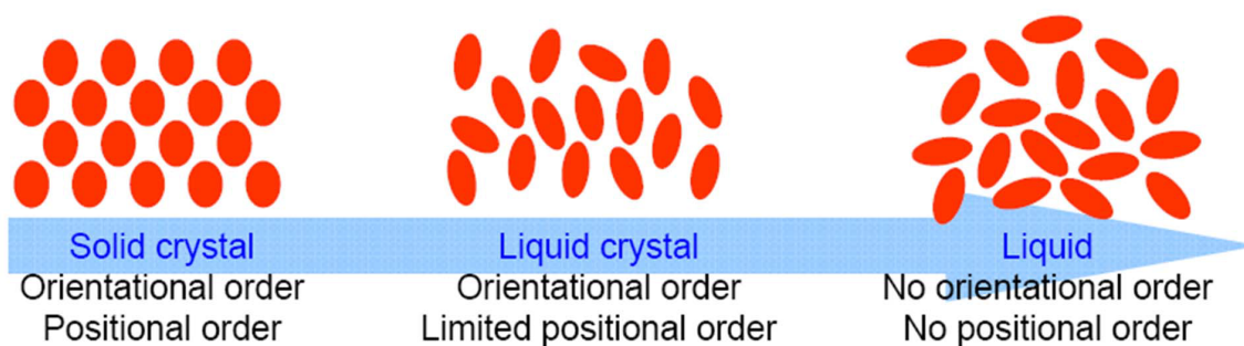
Figure 1.3.: Definition of a liquid crystal based on the orientational and positional order of the molecules. Liquid crystals are in between a solid crystal and a liquid. They have orientational order but no 3-dimensional positional order. (reprinted from [10])
