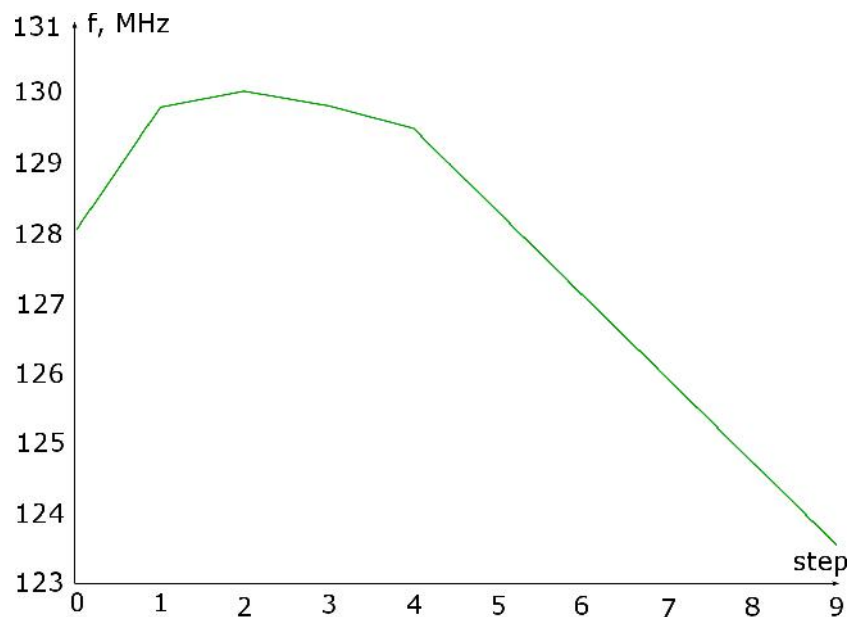
FIGURE 6.8: Expected frequency of the standard inverter based ring oscillator after irradiation obtained from analytical model
