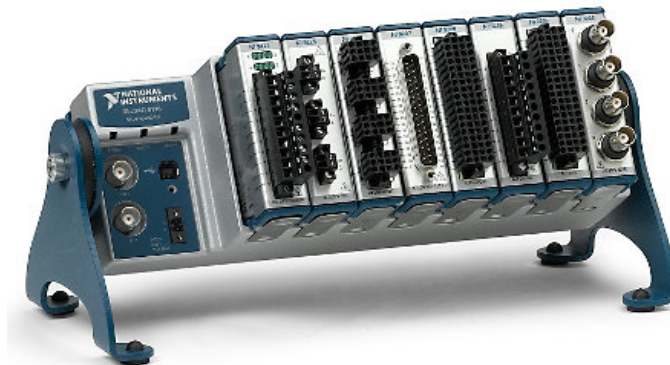
Figure 4.16: National Instruments Chassis type NI cDAQ-9178 with inserted modules [22]
