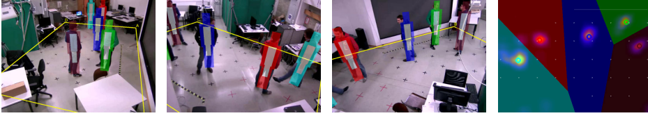
Figure 4.3: Input images with superimposed tracking results (left) and the corresponding occupancy map with Voronoi partitions (right) for t = 1810 of the CHAP dataset. Note that the colors of the Voronoi partitions correspond to the tracker labels.
