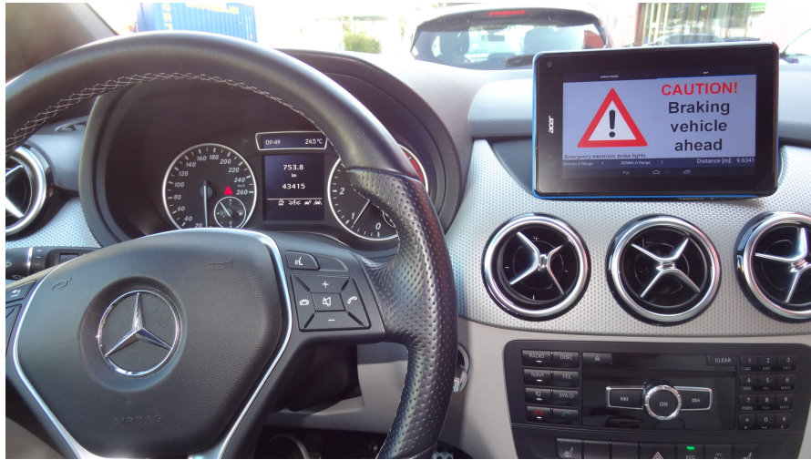
Figure 6.3: Field Test - Dashboard during Emergency electronic brake lights use case
