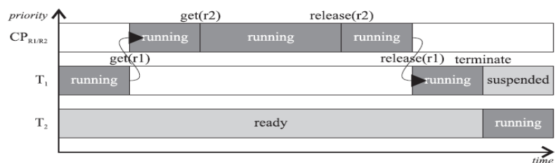
(a) Single-threaded: only one task running. Deadlocks are prevented by priority ceiling
