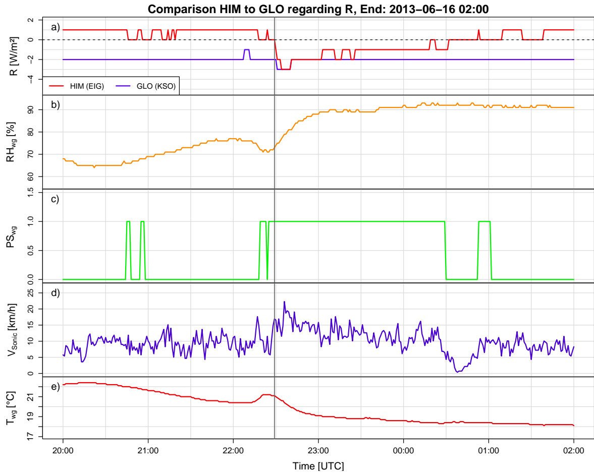
Figure 4.3: Measurements of radiation components at ARAD site Graz/University and meteorological variables (co-located) between 2013-06-15 20:00 UTC and 2013-06-16 02:00 UTC. (a) Radiation R [ \text{W m}^{-2} ] measured at ARAD site Graz/University with sensors for diffuse ( HIM : CMP 21, Eigenbrodt housing, red curve) and global radiation ( GLO : CMP 21, KSO housing, blue curve). (b)-(e) measurements of meteorological variables at co-located TAWES site Graz/University: (b) relative humidity RH_{wg} [%], (c) precipitation sensor PS_{wg} [-], (d) wind speed V_{Sonic} [ \text{km h}^{-1} ], (e) ambient air temperature T_{wg} [ ^{\circ}\text{C} ]. Superscripts near meteorological variables in (b)-(e) indicate location of TAWES sensors (wg: weather garden, Sonic: rooftop, 10 m above ground). Note: Precipitation data is binary (0 or 1) as output of a precipitation sensor is considered instead of absolute amounts. The black dashed horizontal line in (a) marks 0 \text{ W m}^{-2} . The dark gray solid line throughout the graph marks 22:29 UTC when HIM begins to fall.
