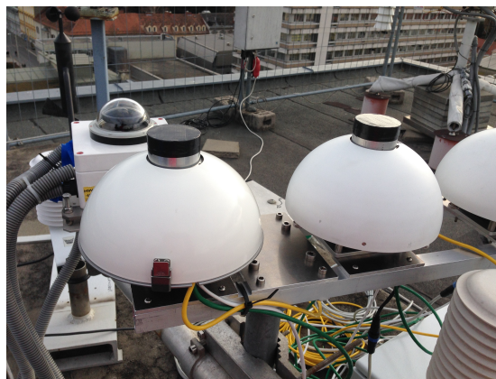
Figure 4.27: Picture of a cover-test on the glass-domes of the reference ( PYRANO A , CMP 21, Eigenbrodt housing, right) and experimental ( PYRANO B , CMP 21, KSO housing, left) instruments with fitted aluminium caps.
