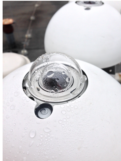
(b) Example for water drops remaining on the outer glass-dome after a spray-test
