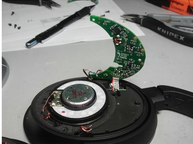
Figure 5.7: Analog filter on the circuit board
