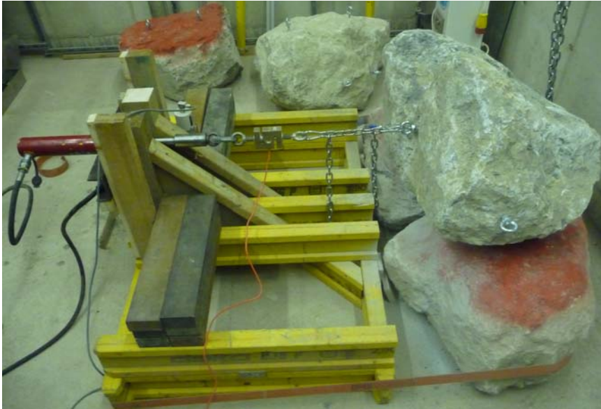
Fig. 15: Layout of pull out trial
