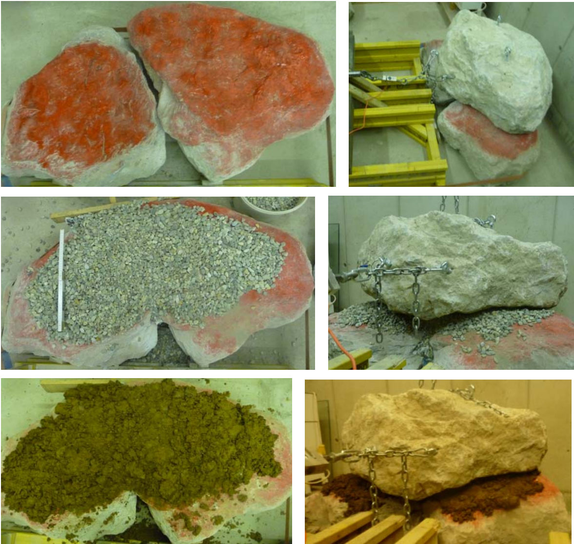
Fig. 16: Pull out trial, block above block, coarse grained material, fine grained material
