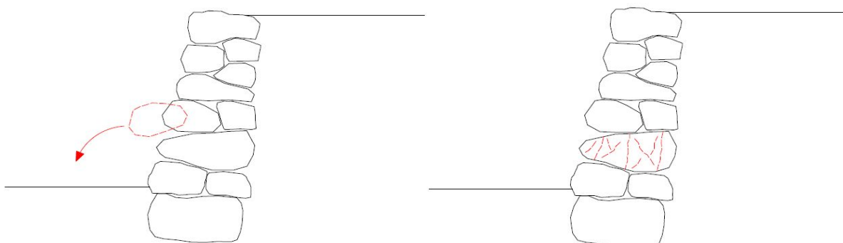
Fig. 25: Sliding of single blocks, material failure
