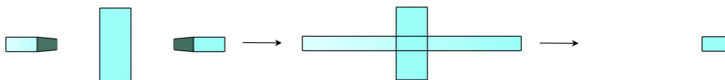
Figure 4.5: Result of the connect-intersection grammar operation. First, an actual intersection has to be created, which is not possible using only splits. Therefore, the two scopes named A1 are connected using connect-convex , and the intersection of this convex hull with the scope named B is used.
