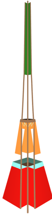
Figure 5.7: The interface of a single leg of the Eiffel Tower: The non-terminals shown in red are connected with the neighbouring leg and fit with the arches. All the non-terminals shown in cyan are connected to form the bottom platform. The orange parts are used for the upper platform support structure. Finally, the green part on the very top is used to only have a single lattice where two legs meet. All these connections are discussed in detail below.
