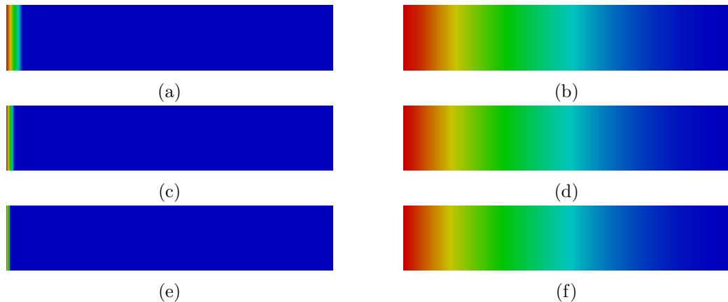
Figure 4.3. Contour plots of the hardening variable \alpha over the halved bar under tensile load for l = 0 mm (left) and l = 3 mm (right) and different mesh sizes: (a)-(b) 20 elements, (c)-(d) 40 elements and (e)-(f) 80 elements. The pictures are taken at u = 1 mm. Note, that the color-coding is not the same for the left and the right pictures.
