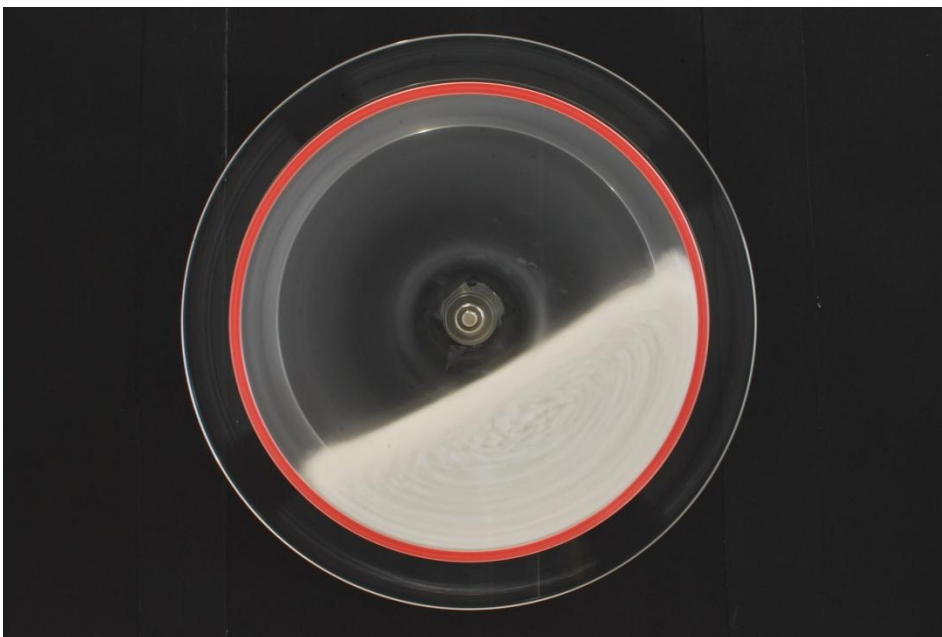
Figure 20: Illustration of an example image of the rotating drum with red fixed points on the edge of the drum in order to increase the contrast and to make the search of circles easier.
