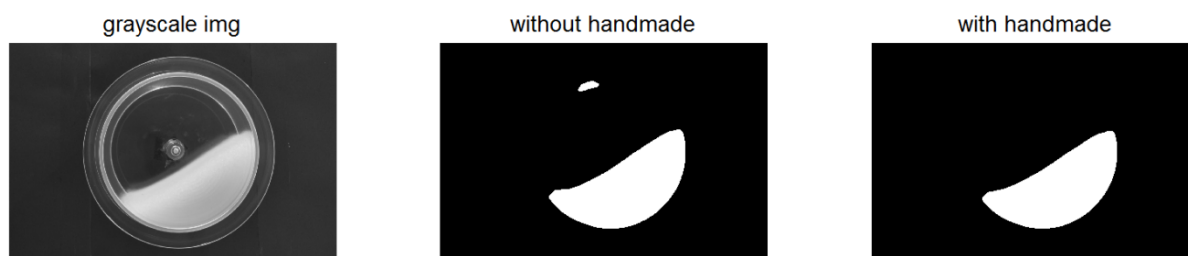
Figure 29: Illustration the advantage of the variable ,handmade' by the appearance of artifacts.
