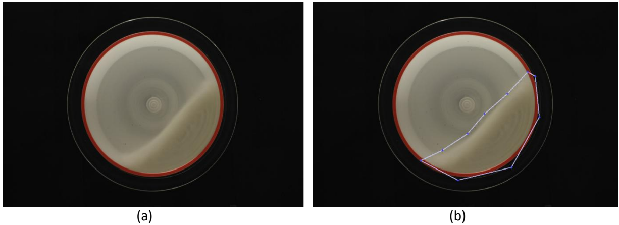
Figure 30: Image of the self-pressed tablet in the rotating drum. (a) without the polygonal line and (b) with the polygonal line.
