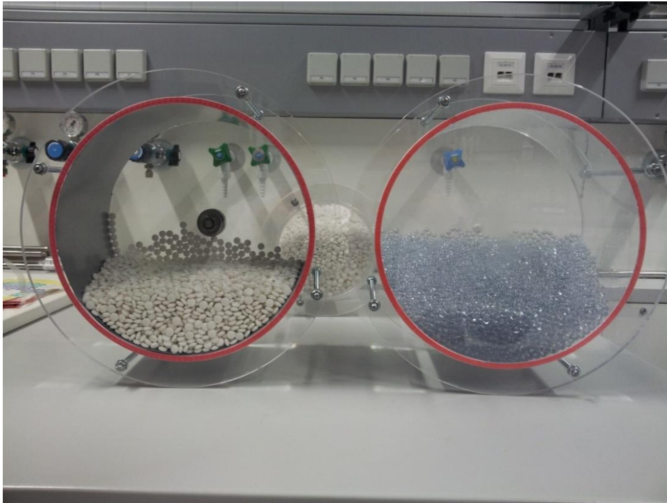
Figure 16: Pictures of the drums used for the experiment. Left hand side: Drum with steel sheet filled with the Thrombo tablets. Right hand side: Drum filled with Silibeads glass spheres.
