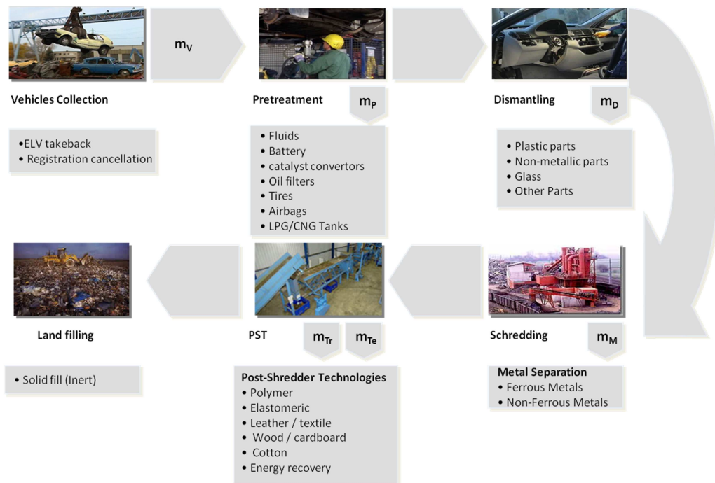
Figure 4-1: Recycling process sequence for end-of life vehicles (Source: MAGNA STEYR)
