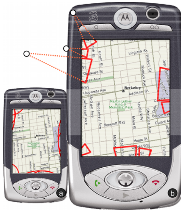
Figure 2.15: Wedges use culled triangles to encode direction and distance to offscreen locations. Compared to Halos (as shown on the small image) Wedges can create much better cues guiding to the hidden locations. [GBGI08]
