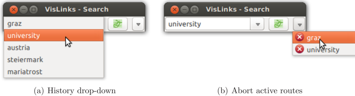
Figure 4.4: The search widget allows initiating new linking processes (a) as well as aborting existing ones (b).
