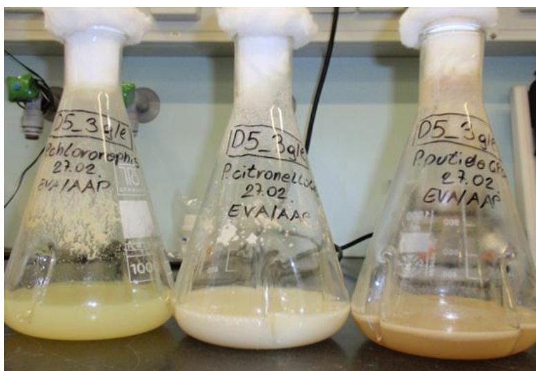
Figure 3. Ps. chlororaphis , Ps. citronellolis and Ps. putida GPO1 on 3 g/L biodiesel after 25 days and continuous feeding (feeding every 3-4 days with 3 g/L). Ps. chlororaphis showed a slightly green culture broth.
