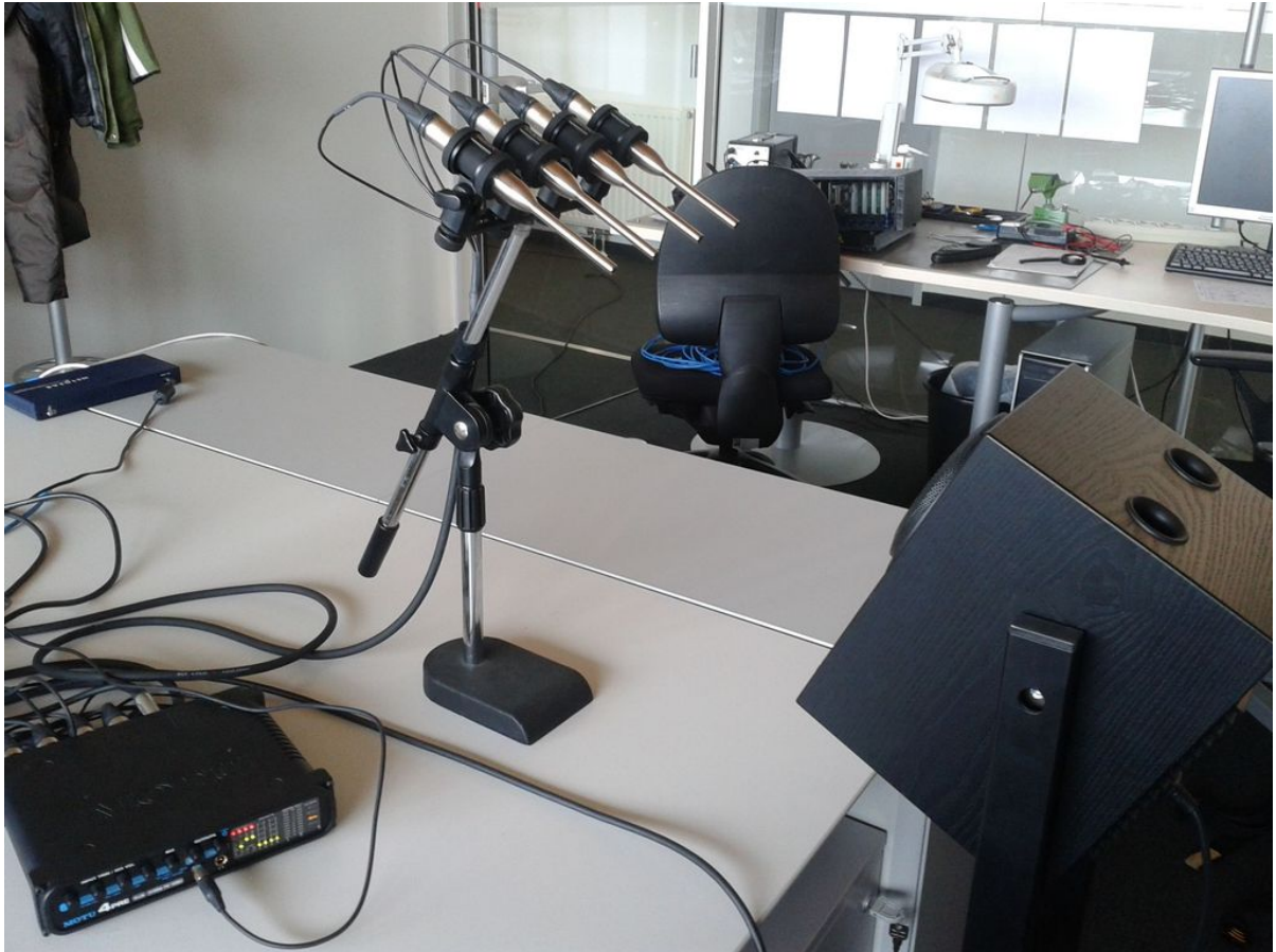
Figure 7.1: Hardware used for the prototype: The four Audix TM1 Plus microphones can be recognized in a linear array combination. In the lower left corner is the MOTU 4pre ASIO interface. The lower right corner shows the Geithain RL906 measurement loudspeaker used for recording the ATF's.
