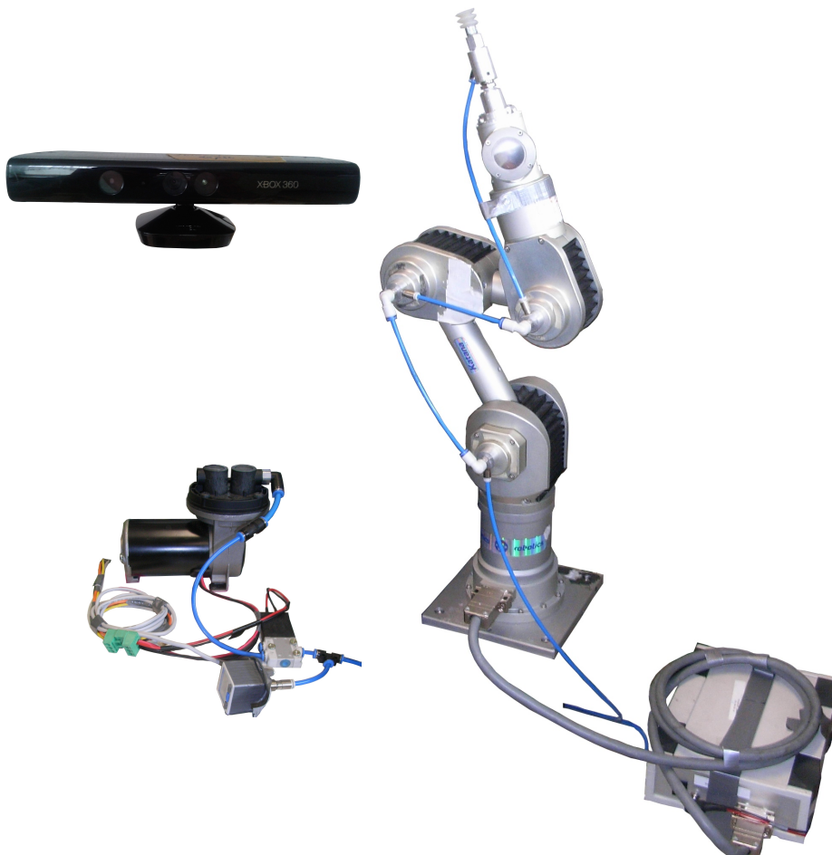
Figure 4.10.: Left: Microsoft Kinect, vacuum pump with valve and pressure sensor; Right: Robot arm with vacuum gripper and arm control box
