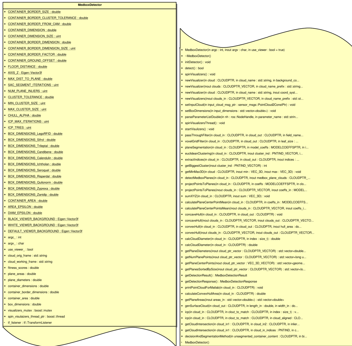
Figure 4.29.: Class diagram of the MedboxDetector class used for the med-box-detector_action_server node
