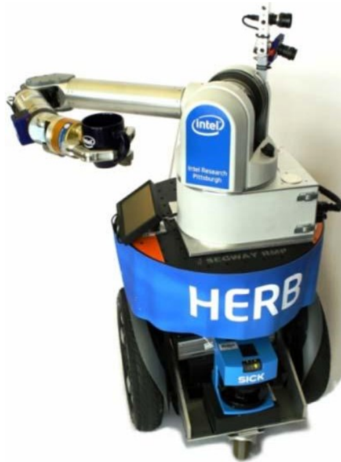
Figure 3.2.: HERB: a platform for personal robotics developed jointly by Intel Research Pittsburgh and Carnegie Mellon University [28]
