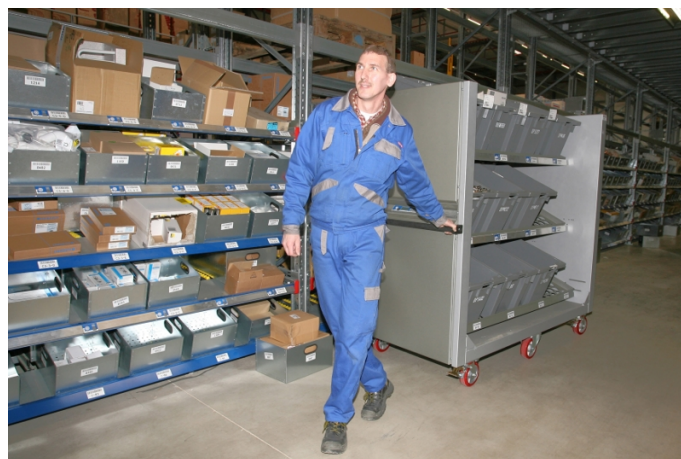
Figure 1.1.: Manual order picking (Photo courtesy of KBS Industrieelektronik GmbH)
