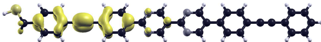
Figure 1.6.3: Iso-density plot of the LDOS of the highest occupied band of a free-standing monolayer with Tour-wire backbone and bi-pyrimidine shifting unit.
