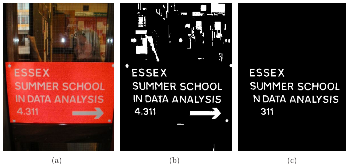
Figure 5.5: The text segmentation approach of Kasar et al. [Kasar2007] on a sample image (a), once computed for the entire image (b) and once computed only within the detected text area locations (c) by the OCVTD algorithm.
