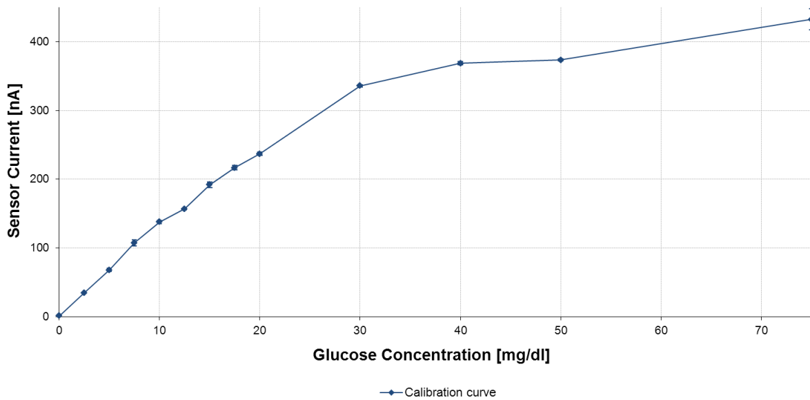
Figure 57: Calibration curve of the BVT AC1.GOD glucose sensor in phosphate buffer.
