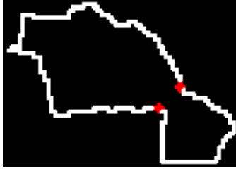
Figure 2.7: Bottleneck detection. Bottleneck pixels (red) of a clump, found by the clump splitting algorithm as defined in Equation 2.19. Reprinted from[43].
