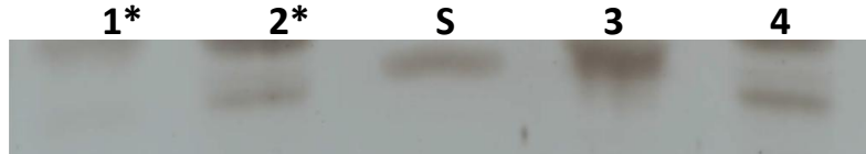
Figure 3. 37: LI-2 iloprost encapsulation efficiency after nebulization with Optineb®-ir, (1) aerosol liposomal iloprost EE ~10%, (2) aerosol free iloprost, (S) iloprost standard, (3) remainder liposomal iloprost EE ~70-80%, (4) remainder free iloprost. Aerosol and remainder samples contain in each case both bands together 4 µg of iloprost. The standard was 2 µg of iloprost. *The sample bands contain together only 0.9 µg iloprost due to insufficient sample volume.
