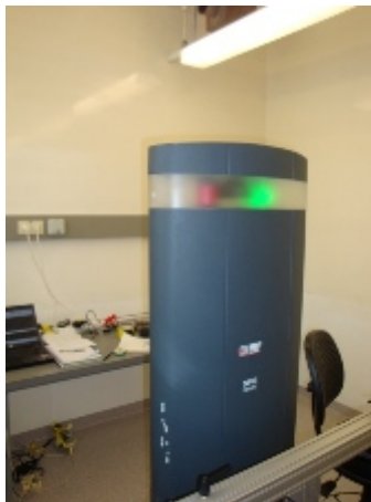
Figure 22: MIRION portal monitor
