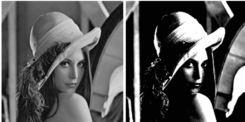
Figure 2.2: An example of a threshold filter with upper and lower bounds (hysteresis threshold) applied to a grey scale image. The left image shows the original input image while the right picture was processed with a hysteresis threshold of t_1 = 100 and t_2 = 150 . The values between those two thresholds remain unchanged.
