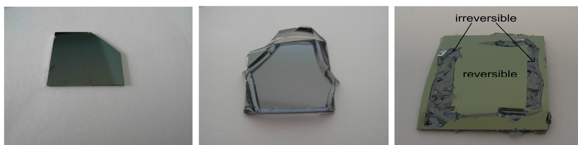
Figure 68: Left; reversible bonding; the PDMS-mold can be peeled off the SiO 2 substrate without leaving any traces. Center; irreversible bonding; the PDMS mold can't be peeled off the SiO 2 substrate. The PDMS rips at the edges before being relieved from the substrate. Right; substrate after peeled off; the PDMS rips before being peeled off the substrate around the edges (irreversible) whereas the center didn't leave any traces (reversible).
