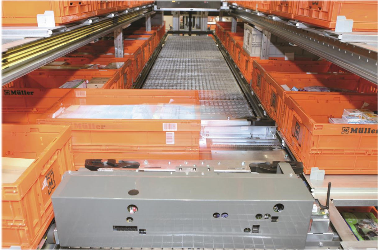
Figure 77: Conductor rails of a KNAPP OSR shuttle system 96
