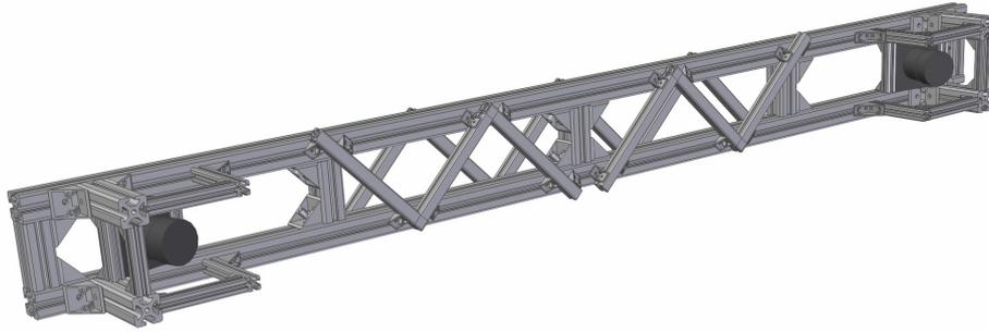
Figure 6.2: CAD model of the camera stand with the cameras mounted at a baseline of  $1600mm$  and an enclosed angle  $\alpha$  of  $30^\circ$ .
