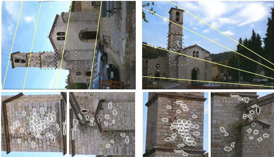
Figure 2.6: VALBONNE: Estimated epipolar geometry and points associated to the matched regions. The image is taken from [MCUP02].
